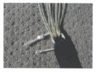
Pass the link through the lines and through the riser again, so that the link forms a doubled loop.
